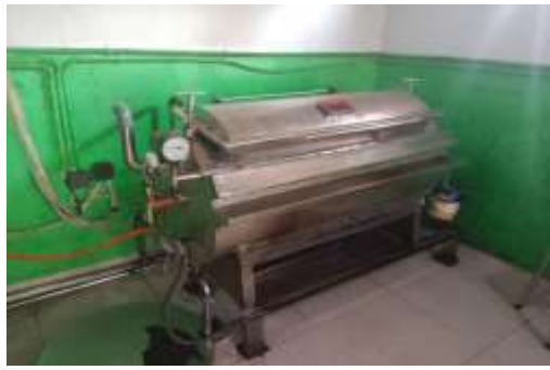
Figure 2. Vacuum Tool for Fruit and Vegetable Chips Production Process
